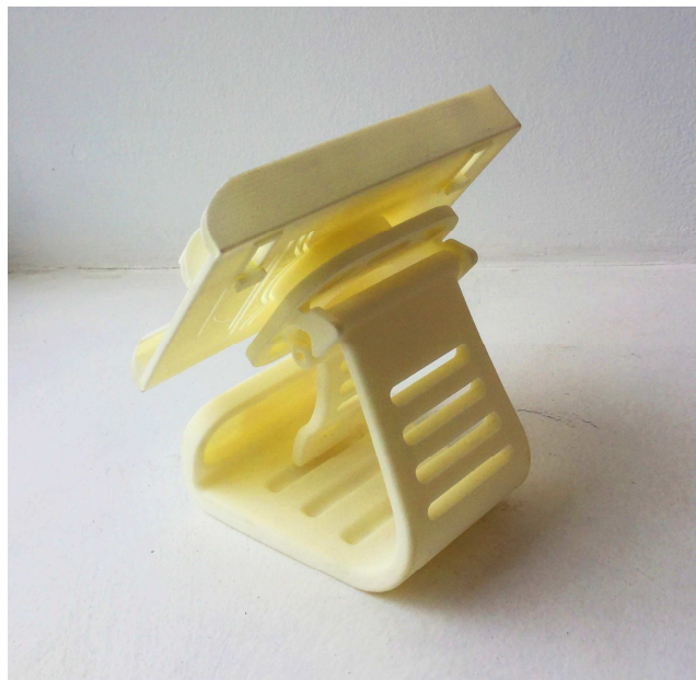
Figure 5. A photo of a 3D printer-designed (SLS technology) cell-phone stand, developed in program SolidEdge.
