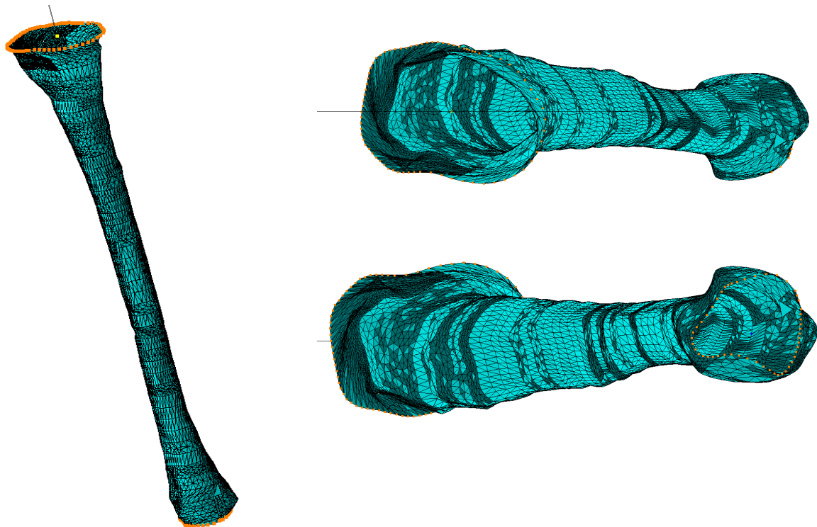
Figure 2. Tibia finite element model in "Lira-SAPR 2013R4" PC: (a) 3D view; (b) top view; (c) bottom view
