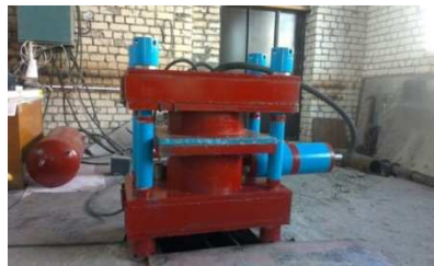
Figure 5. Experimental installation for gas molding with backpressure
