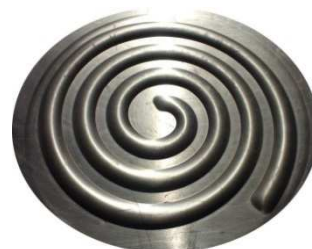
Figure 7. Heat exchanger panel with spiral channel
