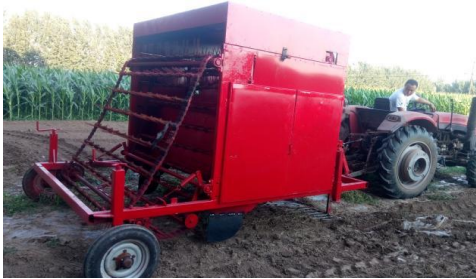
Figure 7. Fields trial of residual film device
