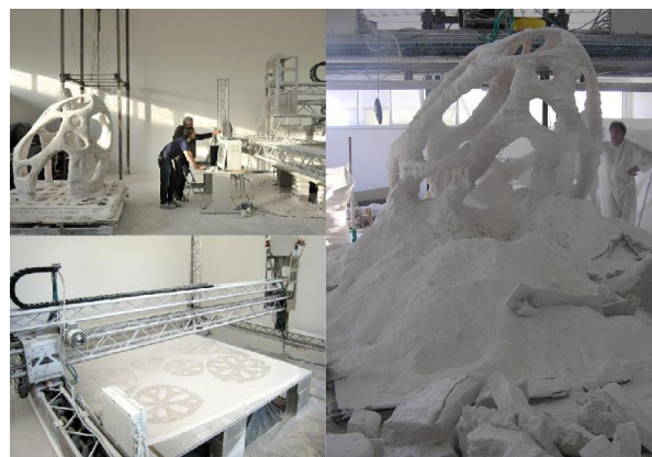
Figure 2. D-Shape 3D Printing Technology.
