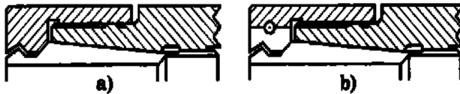
Figure 4. Working principle of spring chuck
