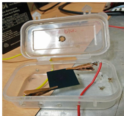
Figure 2. Photograph of Sensor Box with Copper alligator clips.
