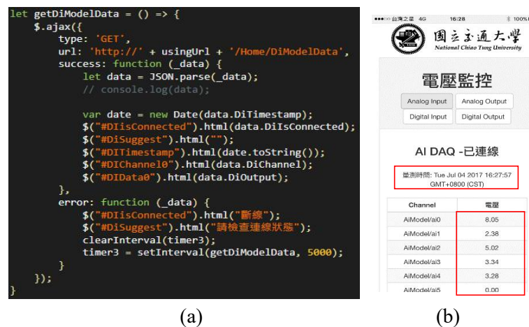
Figure 3. AJAX monitoring interface of mobile browser: (a) AJAX function with jQuery code. (b) Interface of a smartphone.
