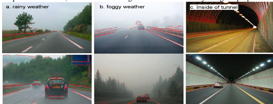
Figure 11. EDLines algorithm with the various conditions.
