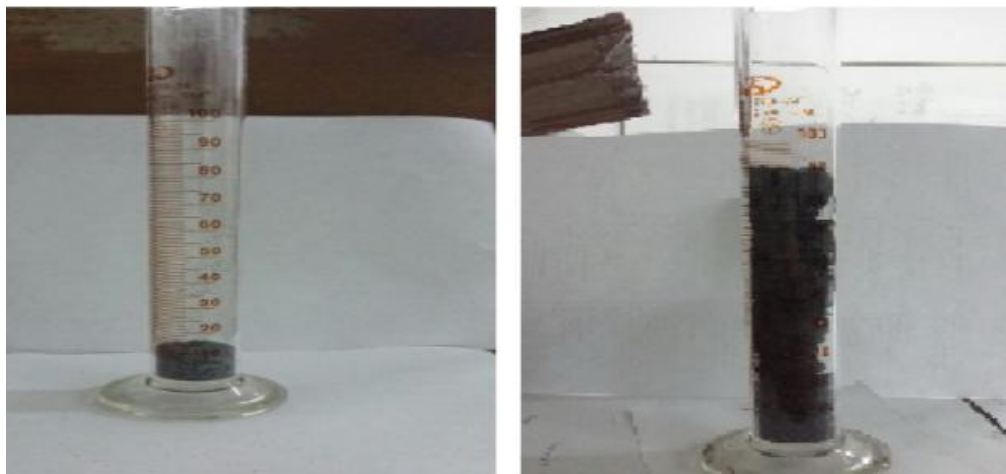
Figure 3. a) mechanical mix before heat treatment b) obtained porous mix after heat treatment.
