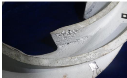
Figure 4. Eroded working surface of a pump impeller.
