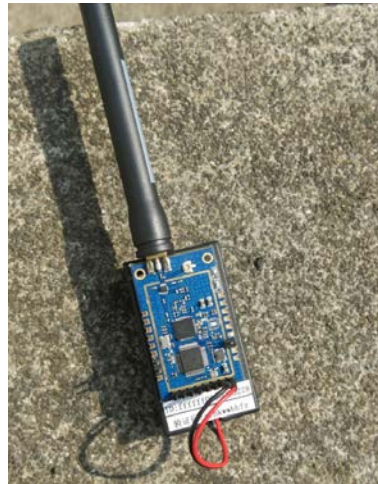
Figure 3. The LoRa module in the test.
