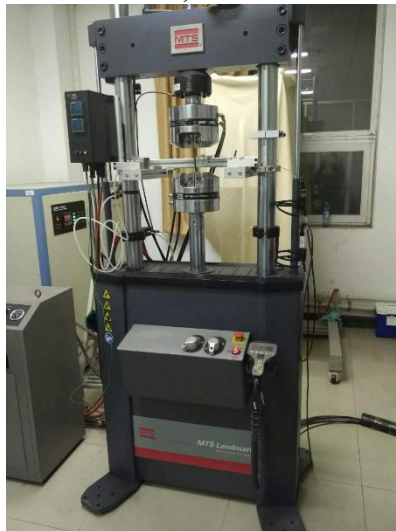
Fig 1. MTS material static mechanical performance testing machine
