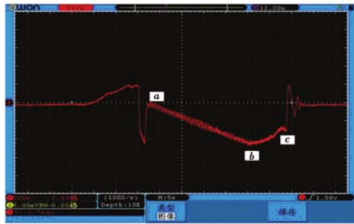
Figure 6. MCU control speed motor output
