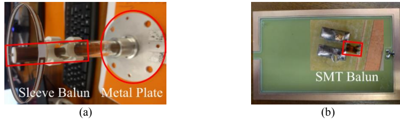
Figure 3. Constructed FSRR antennas: (a) the first prototype with the sleeve balun and metal plate highlighted in red and (b) the adapted prototype with the SMT balun highlighted in red.
