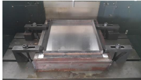
Figure 2: Experiment setup for ISF on CNC milling machine
