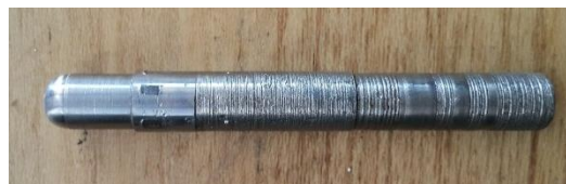
Figure 1: Forming tool for ISF
