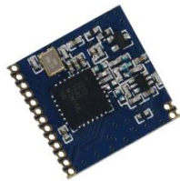
Figure 2. SX1272 LoRa module.
