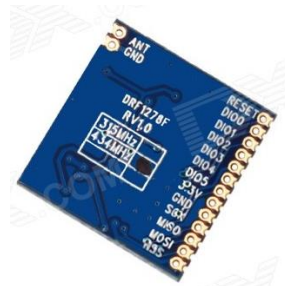
Figure 3. SX1278 LoRa module.
