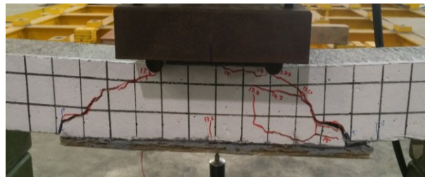
Figure 9. Crack patterns of beam PALF B1.
