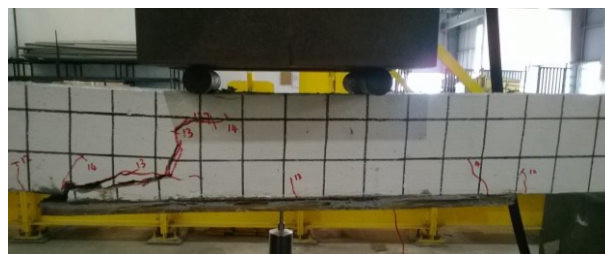
Figure 10. Crack patterns of beam PALF B2.
