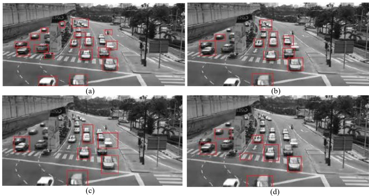
Figure 4. Result for video 2, (a) using optical flow on HD resolution, (b) using optical flow on CCTV video, (c) using foreground detection on HD resolution, (d) using foreground detection on CCTV video.
