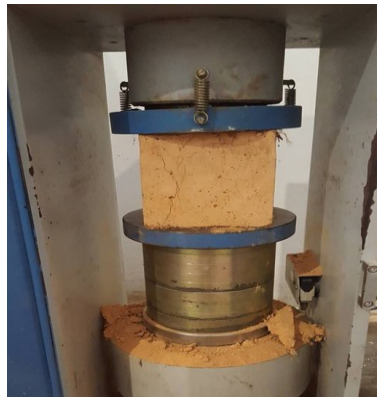
Figure 5. A cube sample being tested for compressive strength
