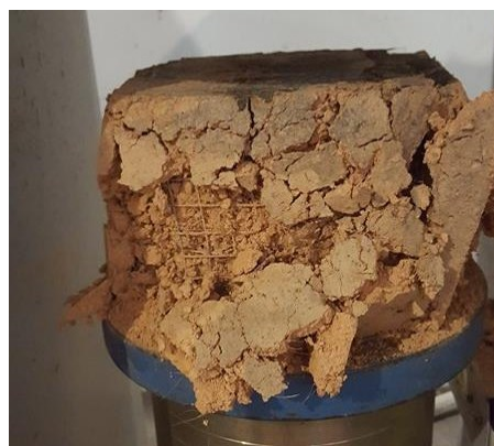
Figure 7. A cubic sample after failure
