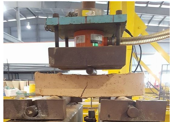
Figure 6. A prismatic sample being tested for flexural strength
