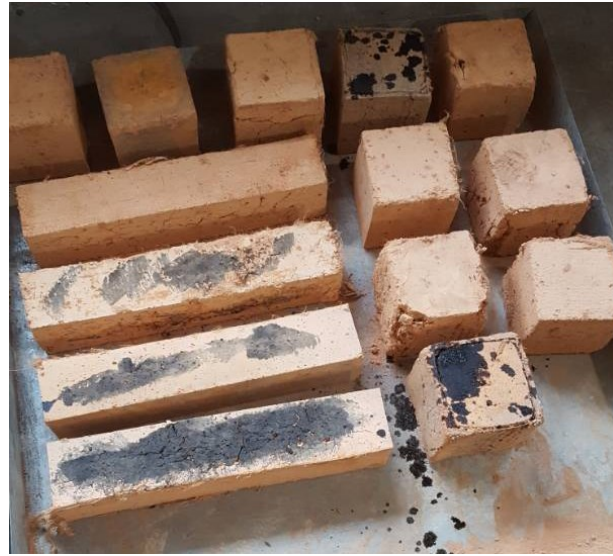
Figure 4. Cube and prismatic samples ready for testing
