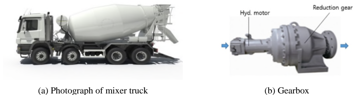
Figure 1. Drum capacity, 8m 3 grade concrete mixer truck and the mixer gearbox with hydraulic motor.
