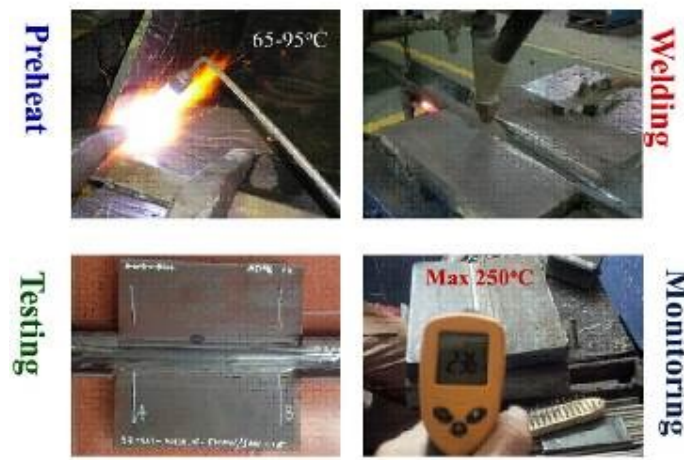
Figure 3. Stages of manufacturing process, from welding, testing and monitoring of joining steel plates
