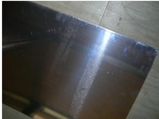
Figure 1: Gold Dust defect in 430 grade Stainless Steel
