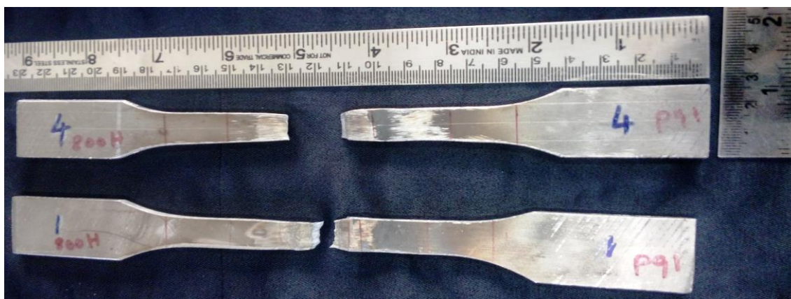
Figure 3. Tensile specimen after testing
