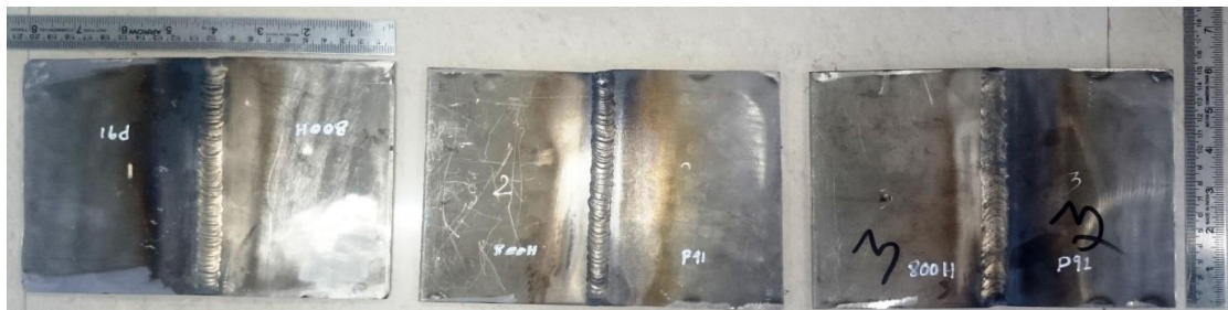
Figure 1. Welded specimens of 9CrMoV-N filler materials
