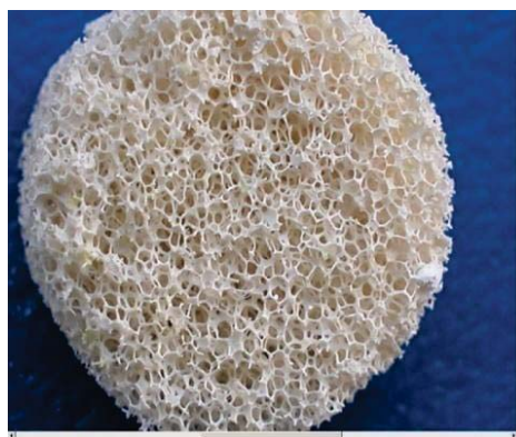
Fig.3 Photograph of porous spun ceramics sintered at 1100°C (sample dia= 8.8mm)
