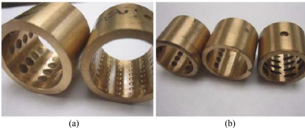
Figure 3. Dimpled bushings (a) machined dimpled bushings (b) etched dimpled bushings
