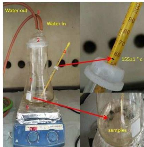
Figure1: Stress corrosion cracking (SCC) test setup [ASTM G36-94]
