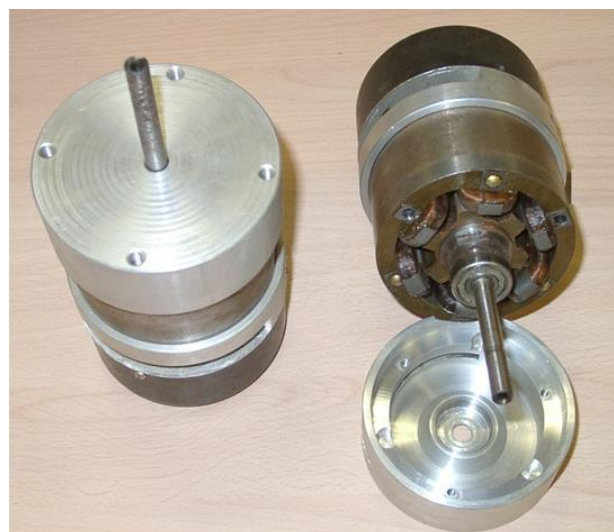
Figure 2. Single-phase SRM
