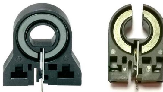
Figure 3. Sensor CSLA1CH prior to and after modification.
