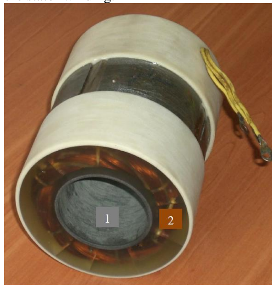
Figure1. The example of using composite materials: 1 is the self-lubricating antifriction material; 2 is the insulating material.
