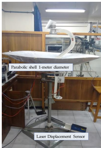
Fig.12. Experimental setup of Reconfigurable parabolic antenna
