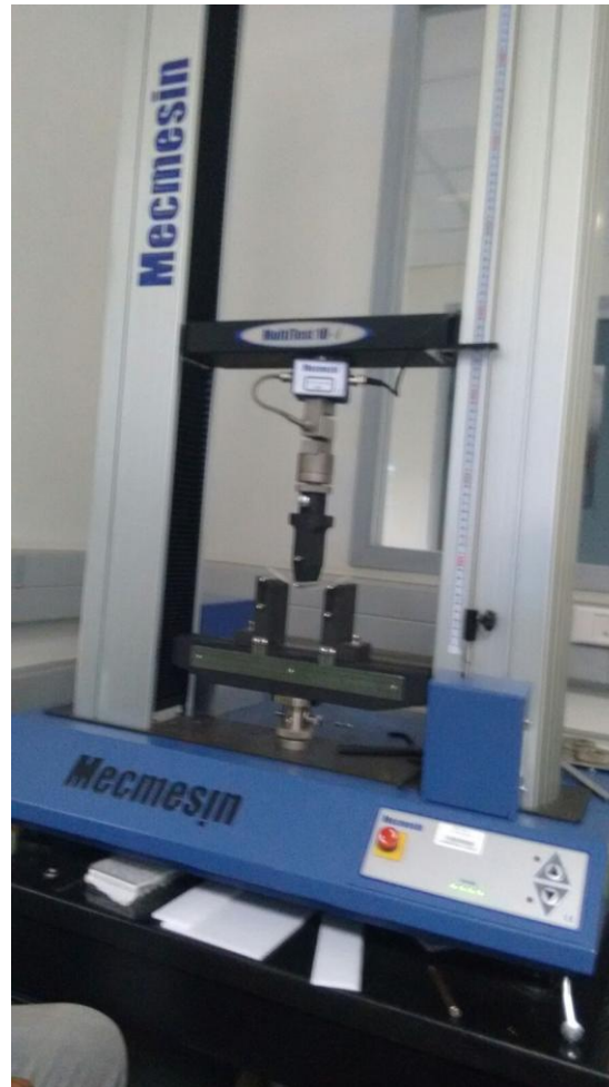
Figure: 2 MECMESIN 3 Point bending machine
