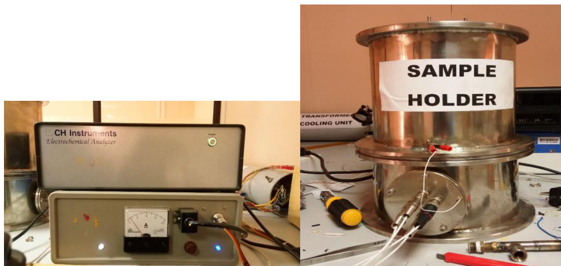
Figure 2: CH Instruments used for impedance measurements and cryostat setup used for placing the sample
