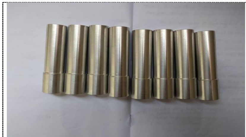
Figure 1. Machined specimens of Al6061
