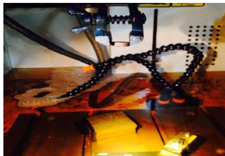
Figure 8. Wear experimental set-up on EDM
