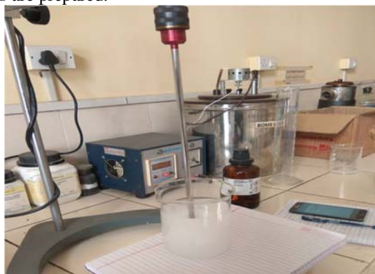
Figure 1. Preparation of the sample fluid using overhead stirrer
