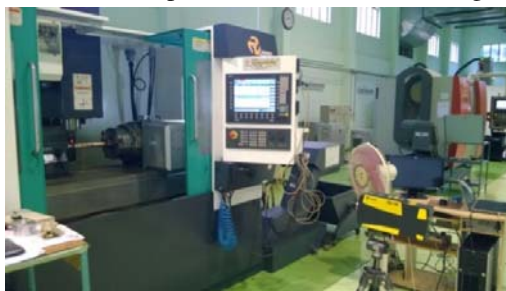
(a) CNC VMC-1050 with A-axis attachment and Poly-Tech 100 Laser Doppler Vibrometer (LDV) (b) Surface Roughness Tester of MITUTOYO Surface Test SJ-301
