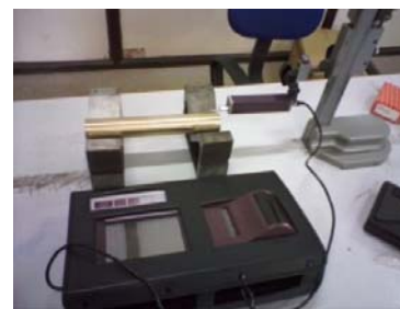
(a) CNC VMC-1050 with A-axis attachment and Poly-Tech 100 Laser Doppler Vibrometer (LDV) (b) Surface Roughness Tester of MITUTOYO Surface Test SJ-301
