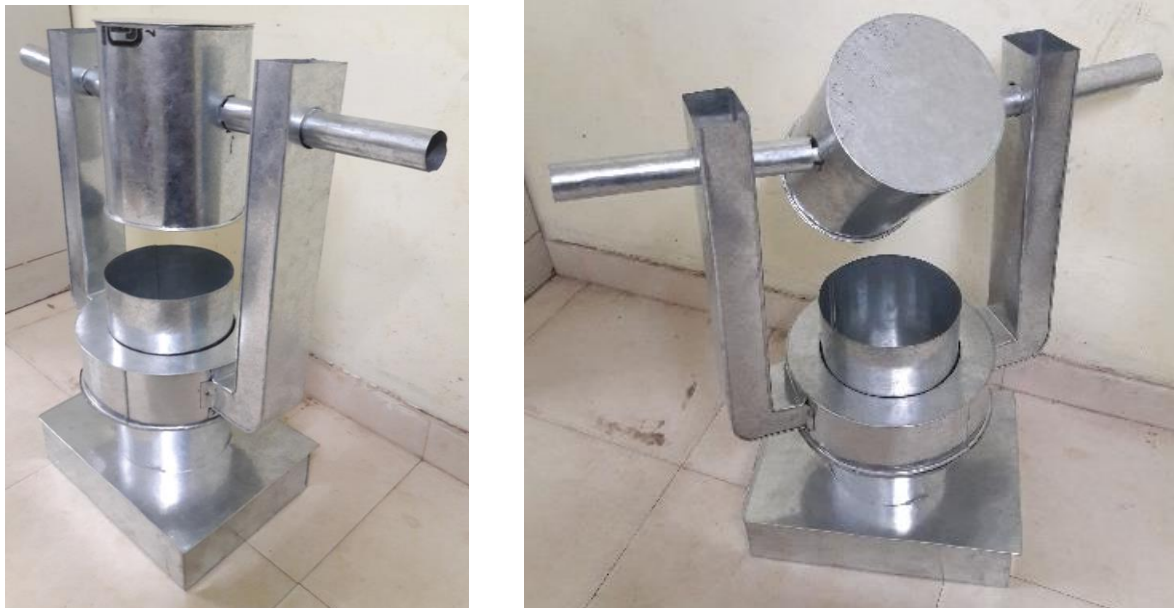
Figure 5 (a) and (b). Different Views of Overall Setup of Fabricated Tilting Rotary Furnace
