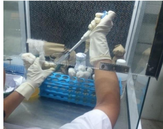
Figure 2 Serial Dilution Technique done to obtain a diluted form to be used in concrete
