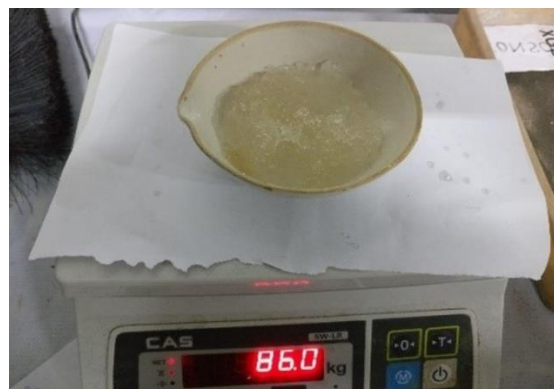
Figure 3 SAP after the addition of Water
