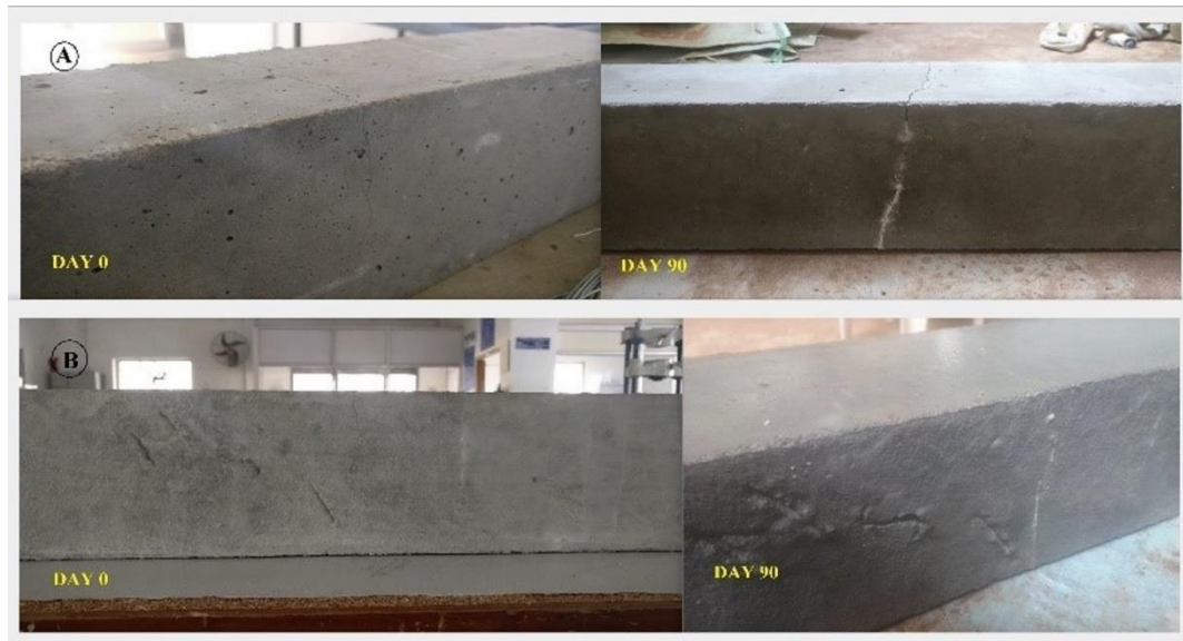
Figure 8 A) represents SAP added Bacterial Specimen with nutrients inside cured in normal water. B) represents Bacterial Specimen without SAP having nutrients inside cured in normal water.
