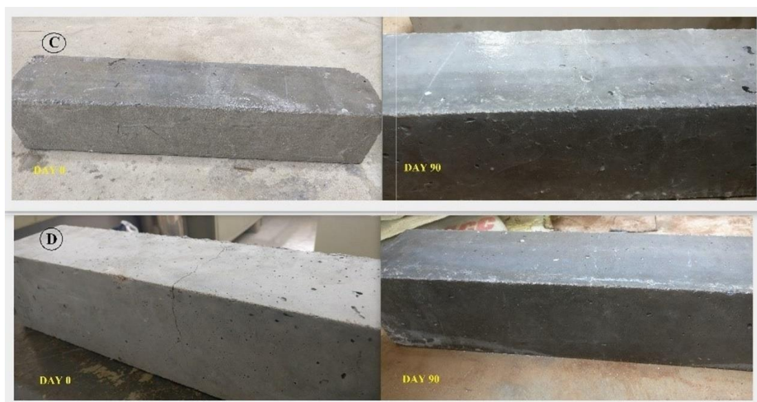
Figure 8 C) represents SAP added Bacterial Specimen cured in nutrients (calcium chloride and urea). D) represents Bacterial Specimen without SAP cured in nutrients (calcium chloride and urea).
