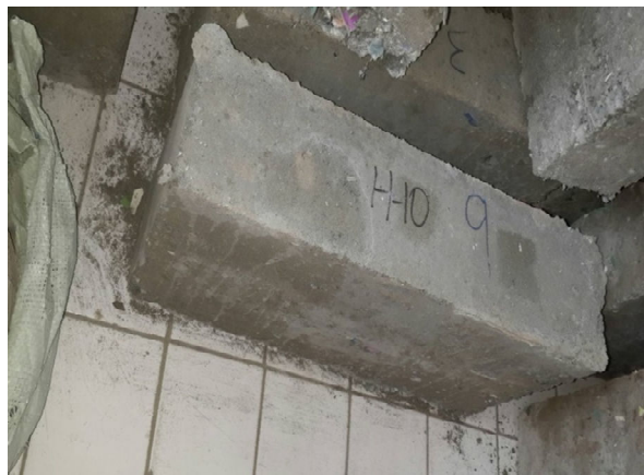
Figure 4. Sample with 10% of HDPE mixture
