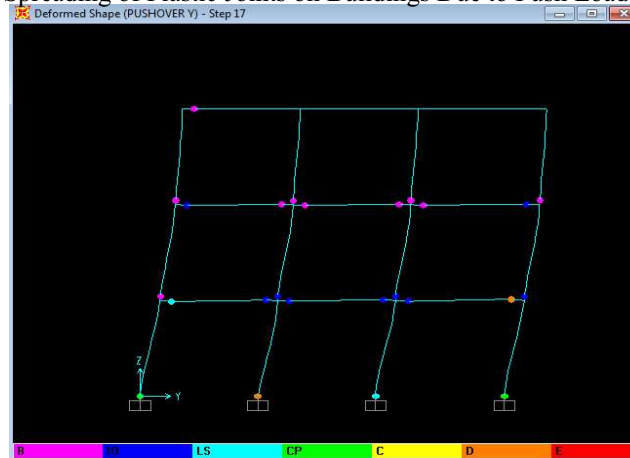
Figure 9. Spreading of Plastic Joints on Buildings Due to Push Load of Y Direction
