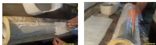
Figure 8. Hand and lay-up mold pattern.
