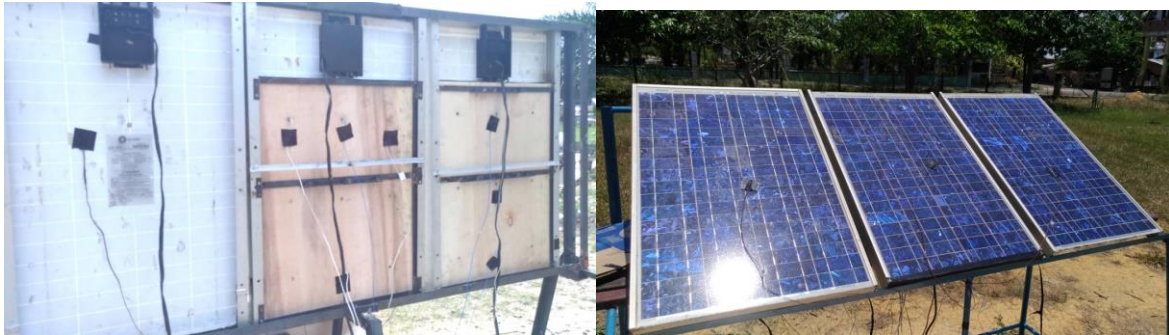
Figure 1. An outdoor experimental setup consisting of a reference PV, PV-PCM1 and PV-PCM2 installed.
