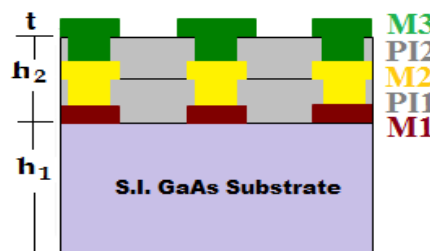
Figure 1. Cross-sectional view of a bonding pad for a multilayer CPW transmission line.
