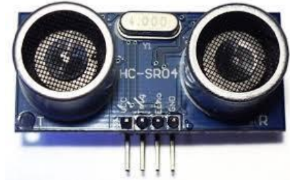
Figure 1. HC-SR04 Ultrasonic Sensor
