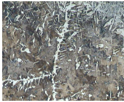
Fig 3. Metallurgical Structure of Failure Sample
