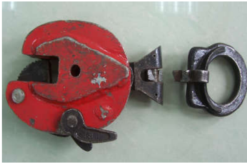
Fig 1. Broken rings
