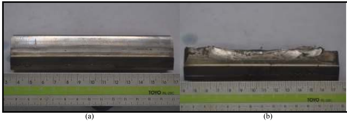
Figure 1. Two gear samples with initial pitting (a) and fractured failed (b)
