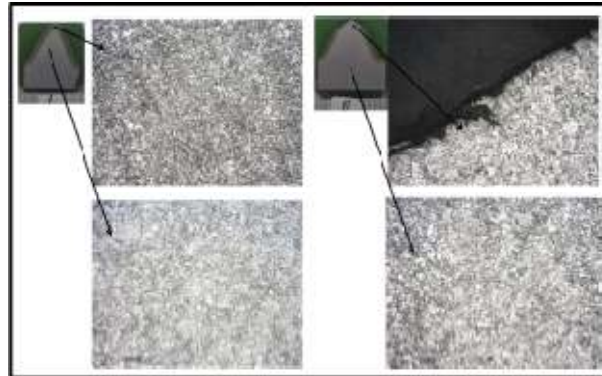
Figure 6. Cros section microstructure of initial pitting gear teeth and fractured gear teeth
