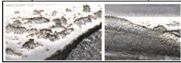
Figure 4. Ridges pattern on macro pitting and rupture crack surface
