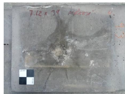
Fig. 9 Crater on the front side after impact
