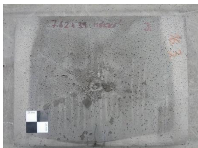
Fig. 8 Projectile stuck in the UHPFRC
