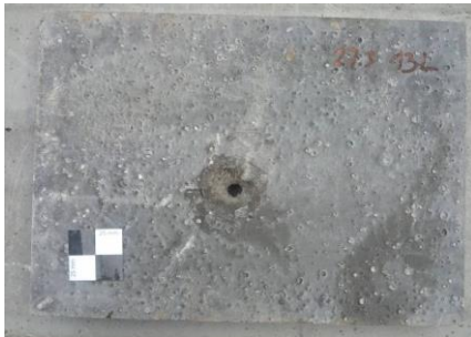
Fig. 4 UHPFRC slab with hole passing through overall thickness
