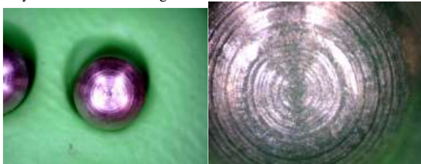
Fig. 2 Traces on new pins
