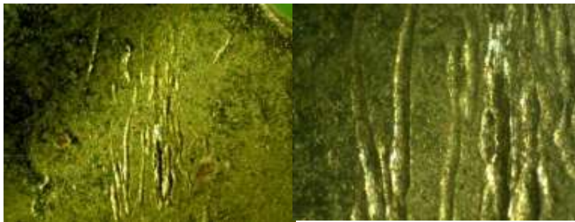
Fig.11 The traces on the keyhole forefront components caused by unlocking guns
