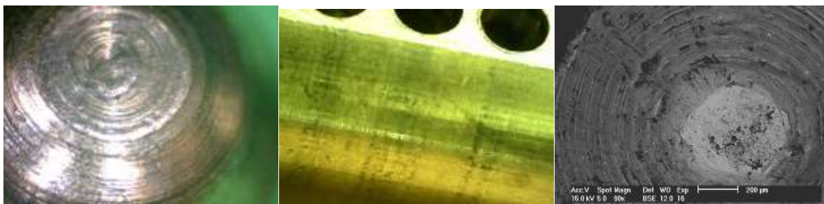
Fig. 3 Traces formed of inserting and removing the key 50 times
