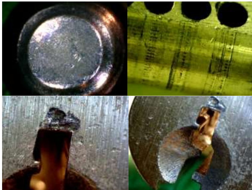
Fig. 5 Traces formed of inserting and removing the key 3000 times
