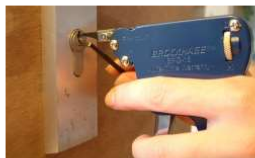
Fig. 7 Unlocking demo with the unlocking gun
