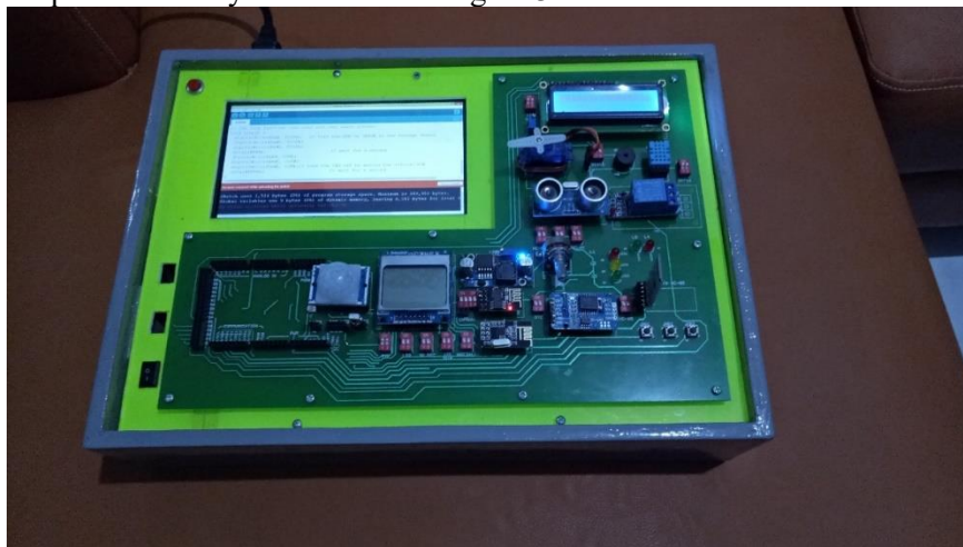
Figure 3. Microcontroller Training Kit Personal Computer Less Physical Form Picture
